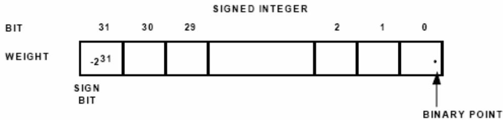
Figure 3.1: 32-bit fixed-point signed integer [20]
