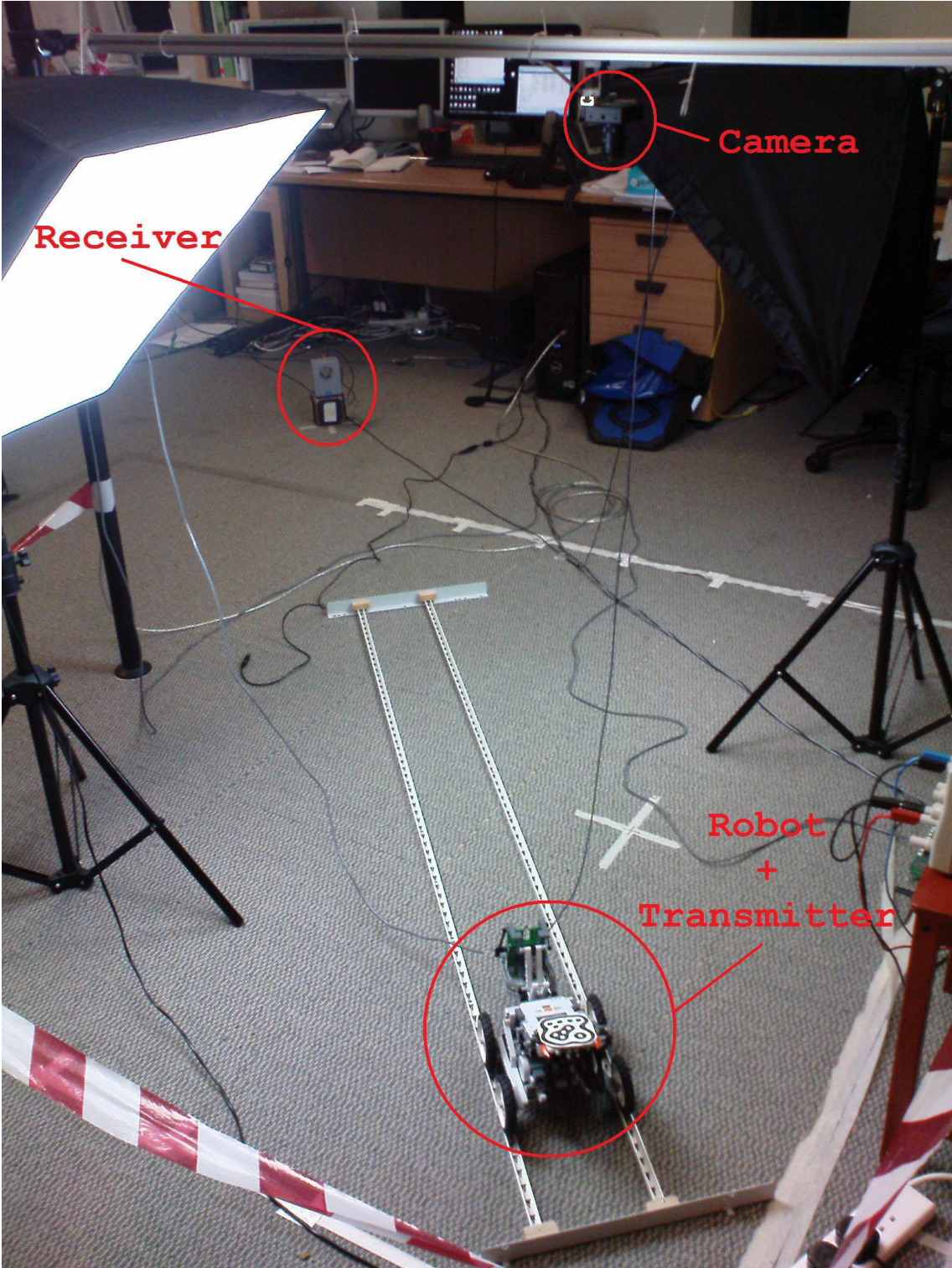
Figure F.3: Doppler data collection setup
